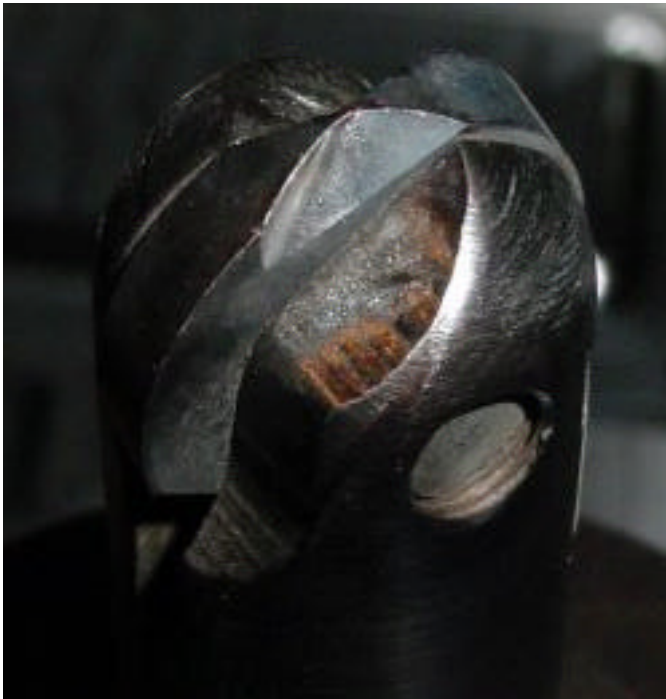
View of Dia 16 Ballnose Insert after Machining
